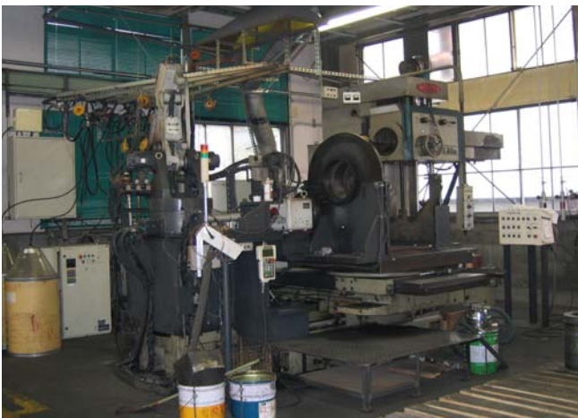
Auto. Compound Welding Machine
